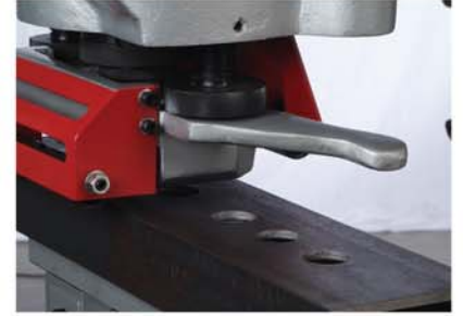
Punching channel flanges and angles
