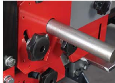
This station allows to cut special bars with special blades such as round, square, channels and many other special profiles
