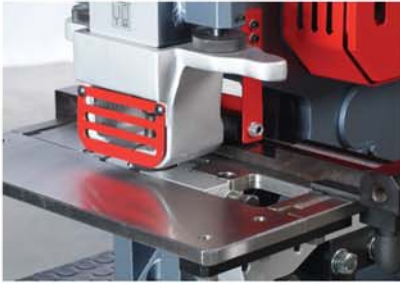
Punching station has max. capacity of \varnothing 27 \times 13 & \varnothing 18 \times 18
