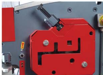
At angle shear station with Z shape aperture, it is possible to make miter shear on angle bars
