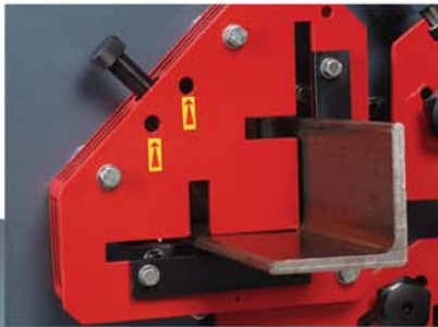
45° miter cut and 90° shearing
